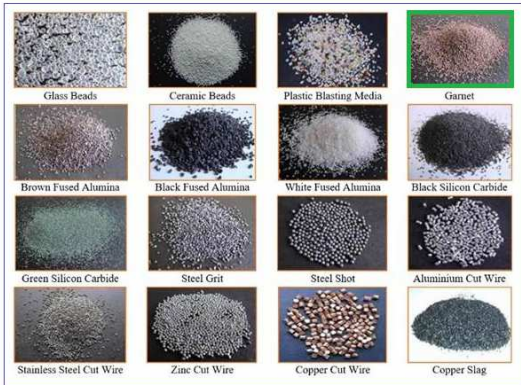
Figure 6. Different types of abrasive used In Abrasive water jet cutting (Alsoufi,2017)
